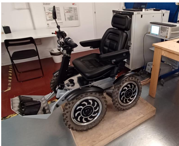
FIGURE 23: CONDUCTED EMISSIONS TEST SETUP
