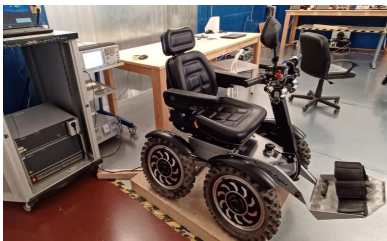
FIGURE 26: VOLTAGE FLUCTUATIONS AND FLICKER TEST SET-UP
