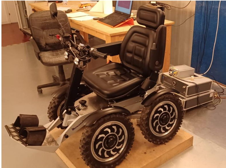
FIGURE 44: VOLTAGE DIPS AND INTERRUPTIONS TEST SET-UP
