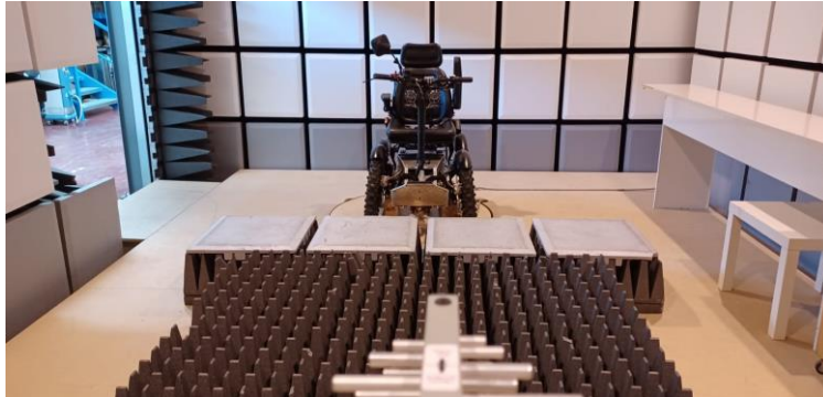
FIGURE 46: RF ELECTROMAGNETIC FIELD TEST SET-UP
