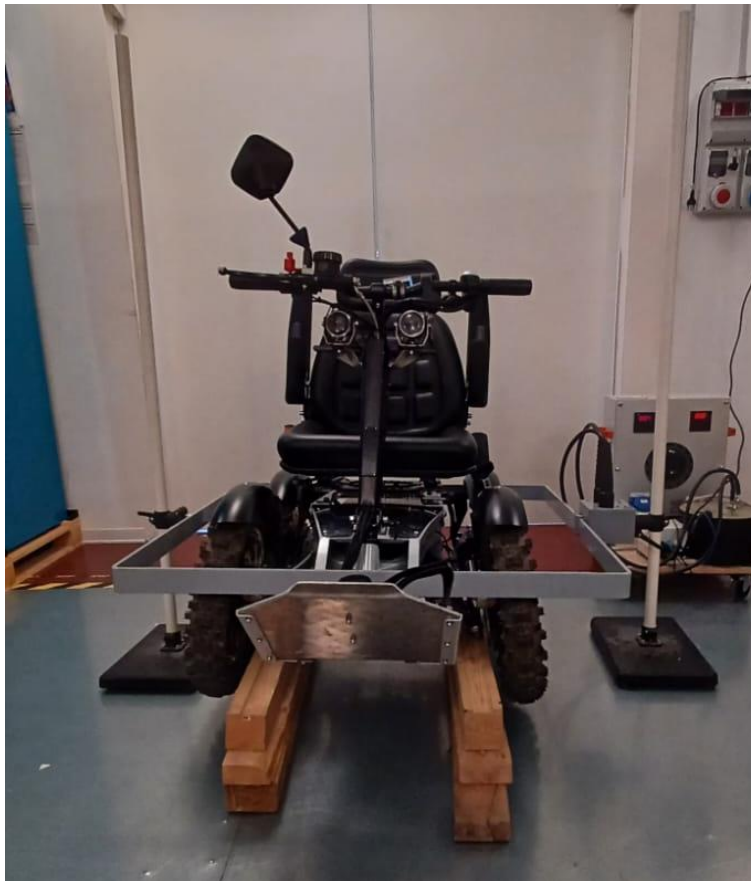
FIGURE 45: MAGNETIC FIELD TEST SET-UP
