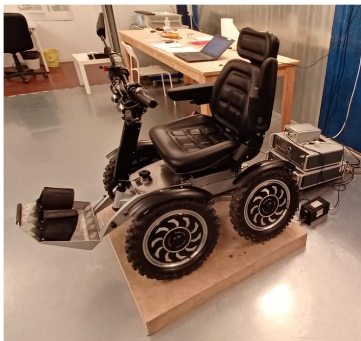
FIGURE 43: RF CONDUCTED DISTURBANCE AC POWER PORT TEST SET-UP
