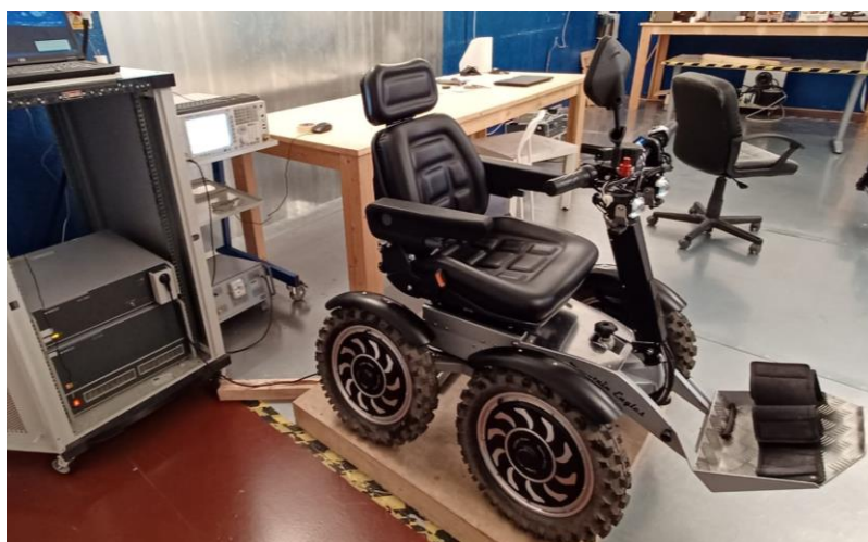
FIGURE 25: HARMONIC CURRENT EMISSION TEST SET-UP
